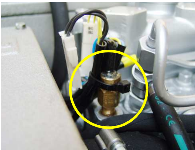
Fig. A.3.7-1: Thermo-switch at cylinder head
