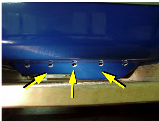
Fig. A.3.5-2: Sound cover drillings
