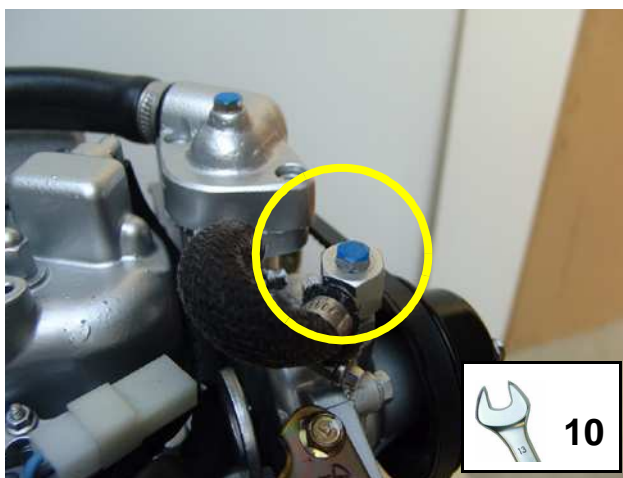
Fig. D.6-1: De-aerating screw - water pump
