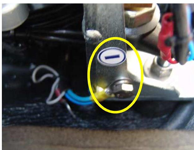
Fig. A.3.6-3: Connection starter battery minus cable
