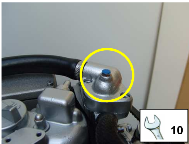
Fig. D.6-2: De-aerating screw - thermostat housing
