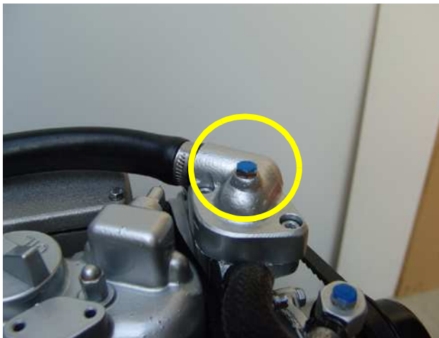
Fig. A.3.3-10: Ventilation screw thermostat housin
