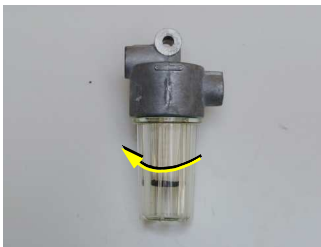
Fig. D.4.2-2: Fuel filter
