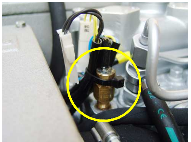
Fig. C.1-1: Thermo-switch at cylinder head
