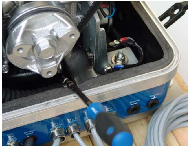
Fig. H.3-3: First hose clamp
