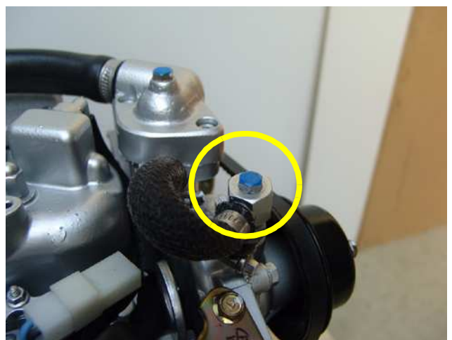
Fig. A.3.3-9: Ventilation screw cooling water pump
